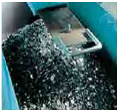
Punch chips generated by bolt hole drilling
